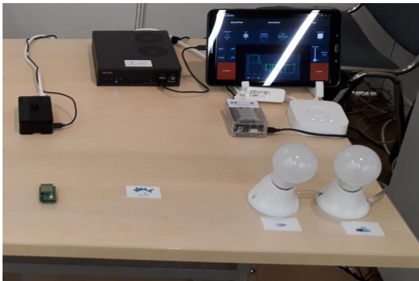
FIGURE 8: IIOT TESTBED INFRASTRUCTURE, SHOWING THE CONTROLLER NODE, IOT GATEWAYS, SMART SENSOR AND ACTUATORS (SMART LIGHTS) AT THE EUCNC 2018 EXHIBITION
