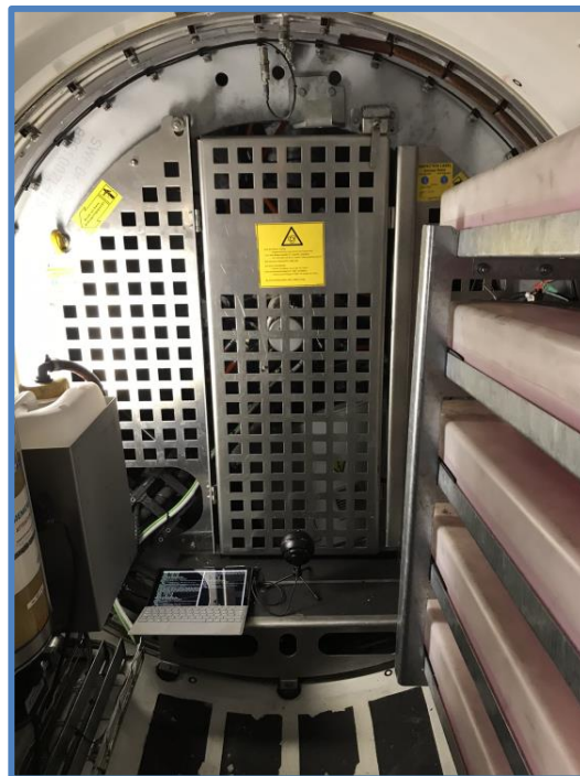
FIGURE 5: MICROPHONE (AT THE BOTTOM OF THE DOOR) INSTALLED IN WIND TURBINE
