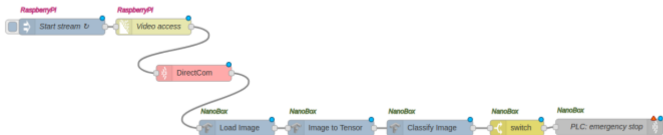
FIGURE 98: IOT APPLICATION FLOW FOR OIL LEAKAGE DETECTION.
